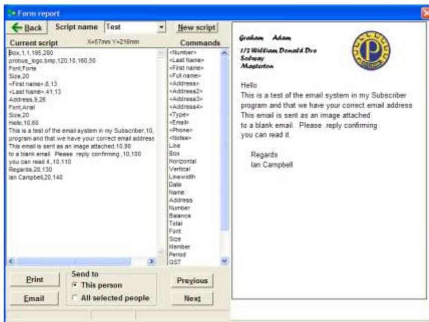
The left hand box contains the script with commands for creating the output on the right, the middle box contains the possible keyword.
